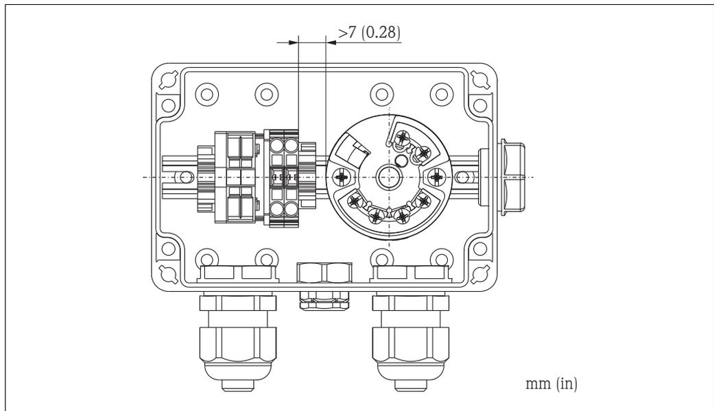
**i** A distance of > 7 mm (> 0.28 in mm) must be maintained between the terminal strip and the TMT182 temperature head transmitter.
