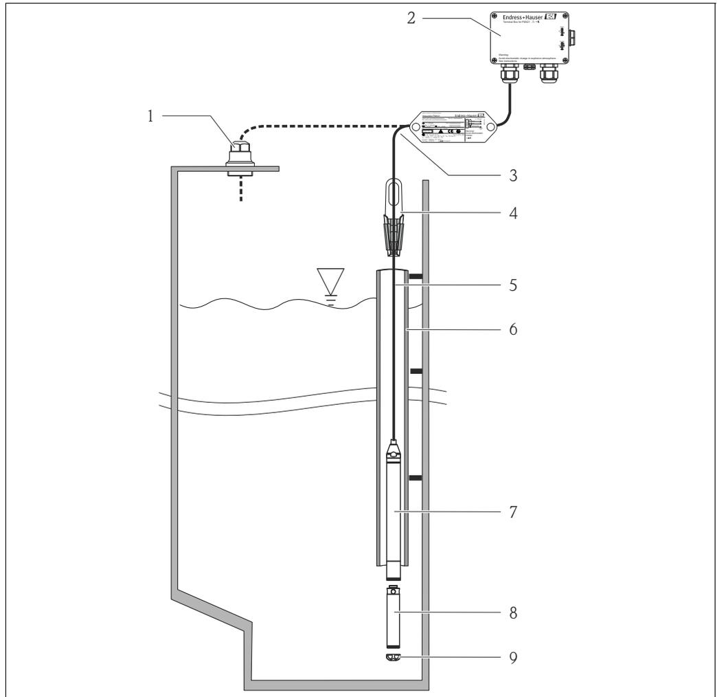
Installation examples, here illustrated with FMX21 with an outer diameter of 22 mm (0.87 in)
