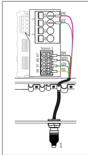
40 M12 plug-in connection (e.g. at sensor module)
