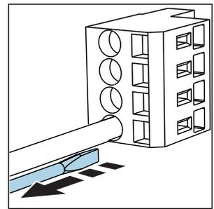
*Remove the screwdriver (closes the terminal)*
