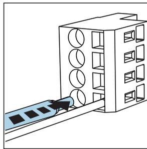
*Insert the cable until the limit stop*
