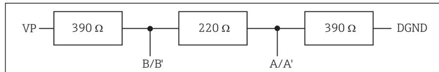
69 Structure of the internal terminating resistor
