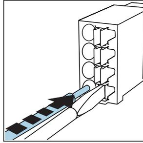
*Insert the cable until the limit stop*
