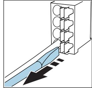
*Remove the screwdriver (closes the terminal)*
