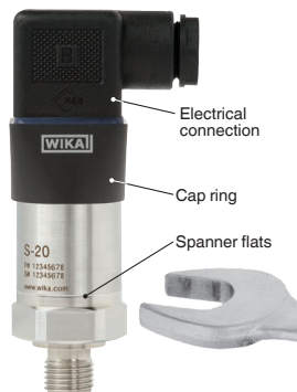
Model S-20 without cooling element
