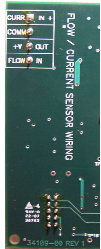
Figure 3-12: Flow/current input signal board and sensor cable leads
